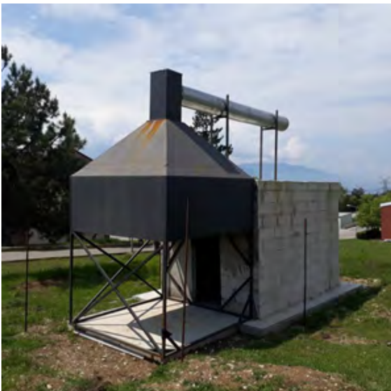
Standard Fire Room Test Mechanism
